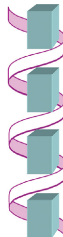
Figure 4. Schematic representation of 1-D POSS arrays encapsulated within the helical st -PMMA cavity.
